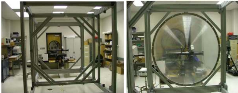
Fig. 4 Lens support frame and metering structure (left) and third BBM lens mounted in frame and metering structure (right). One can see the 60 cm mirror in the back of the left photo.
