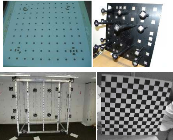
Figure 11: Different testfields used to calibrate the range imaging camera. None of them was usable for the calibration of the SR-2.
