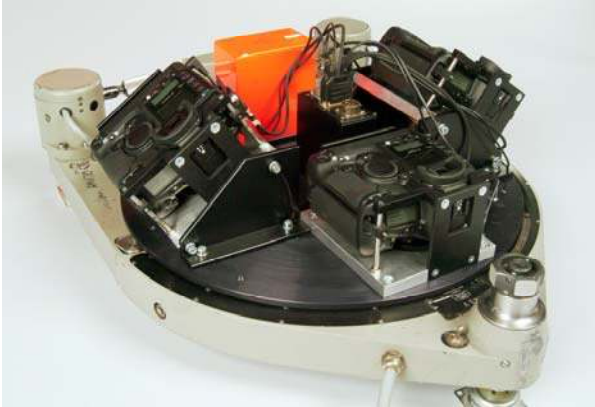
Fig 1. DLR 3K-camera system consisting of three Canon EOS 1Ds Mark II, integrated in a ZEISS aerial camera mount
