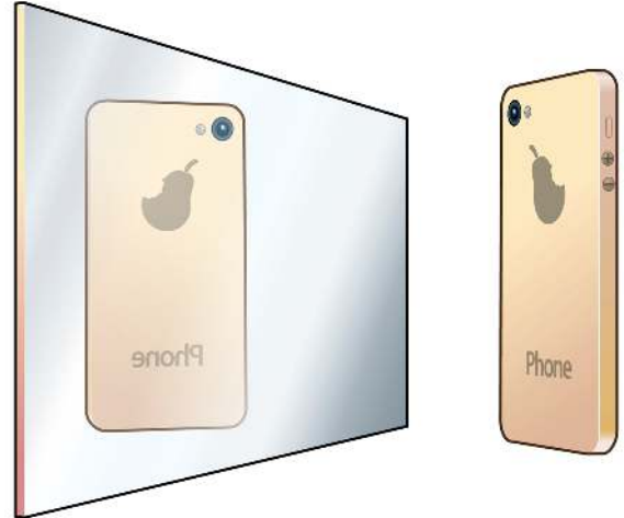
Fig. 1: An illustration of a potential application of the mirror-based IMU-camera calibration procedure for a smartphone, which has an embedded IMU and a camera. The figure shows a smartphone (to the right) and its mirror image (to the left). The logo of the phone (pear) can be considered as an object whose features’ reflections in the mirror are in the camera’s field of view.
