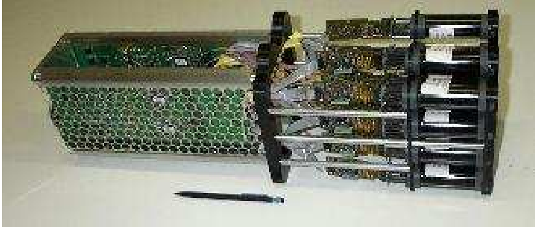
Fig. 1. A camera drawer with its 16 PMTs, the individual HV supplies for each PMT, the two 8-channel acquisition cards and the control/interface card.
