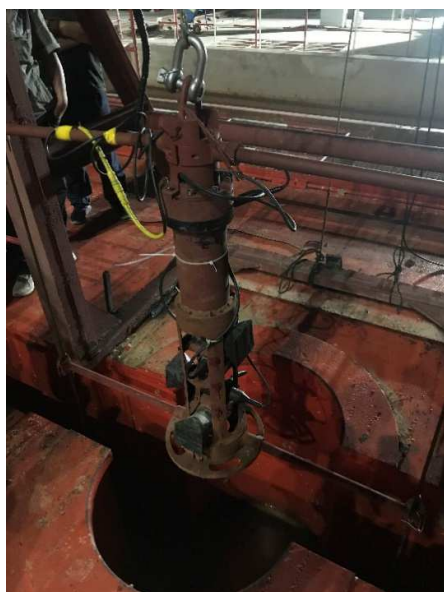
Figure 1. ULISSD used to log the central-air-return shaft.
