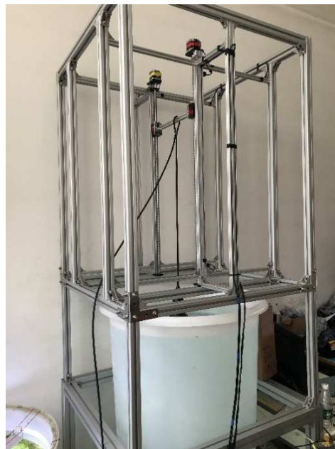
Figure 6. Longitudinal-ultrasonic-transducer error-calibration-test platform with a height of 1500 mm.
