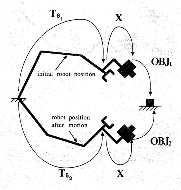
Figure 1.3. If the robot is moved from position  $T_{6_1}$  to  $T_{6_2}$  and the position of the fixed object relative to the camera frame is found to be  $OBJ_1$  and  $OBJ_2$ , respectively, then the following equation is obtained:  $T_{6_1} \times OBJ_1 = T_{6_2} \times OBJ_2$ , where X is the unknown transform representing the camera mounting position relative to the robot wrist frame.
