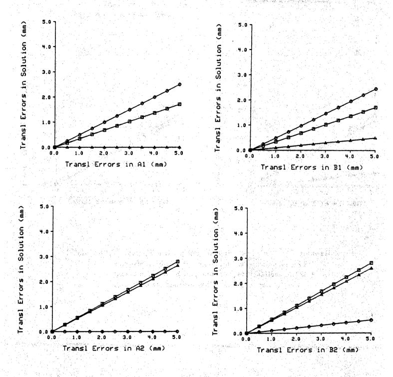
Figure 6.1. Translational noise sensitivities due to translational perturbations of robot motion measurements and sensor motion measurements. Errors due to perturbations in x, y, and z directions are marked by  $\Box$ ,  $\bigcirc$ , and  $\triangle$ , respectively.
