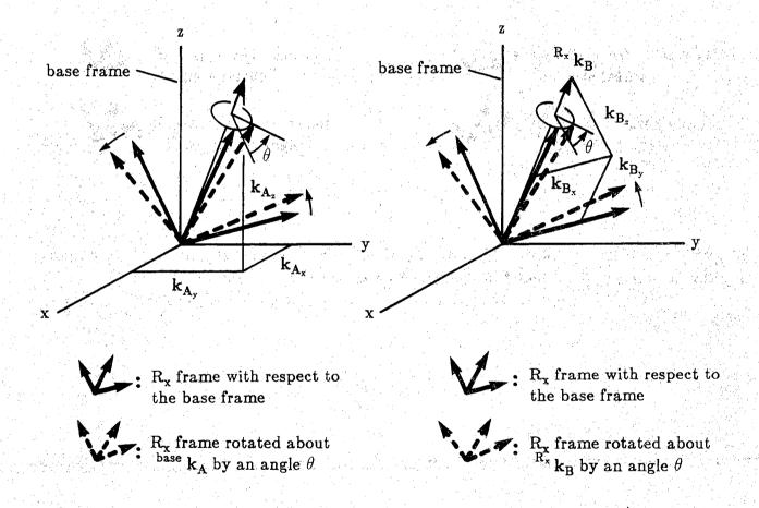
Figure 3.1. Rotating  $R_x$  about base  $k_A$  by  $\theta$  is equivalent to rotating  $R_x$  about  $R_x$   $k_B$  by the same angle.  $k_A$  is the axis of rotation of A and  $k_B$  is the axis of rotation of B in the homogeneous transform equation AX = XB.
