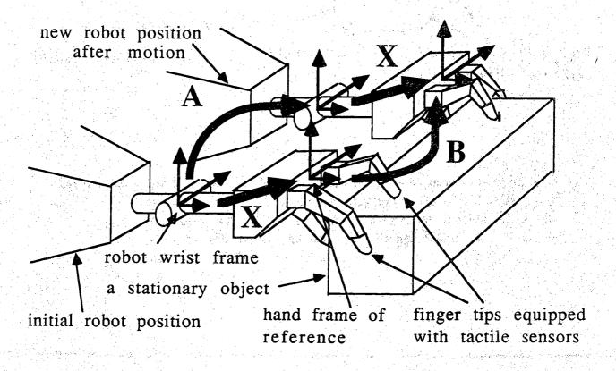
Figure 1.2. Finding the mounting position of a robot hand equipped with tactile sensors, by solving a homogeneous transform equation of the form AX=XB, where A is the robot motion, B is the resulting motion of the hand coordinate frame, and X is the mounting position of the hand.
