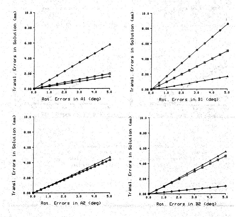
Figure 6.2. Translational noise sensitivities due to rotational perturbations of robot motion measurements and sensor motion measurements. Errors due to perturbations about the x, y, and z axes are marked by  $\Box$ ,  $\bigcirc$ , and  $\triangle$ , respectively.
