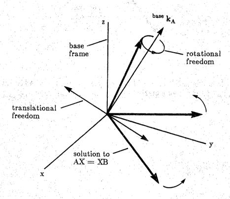
Figure 3.2. The rotational and translational degrees of freedom of the solution to AX = XB. The frame in the figure can rotate about base  $k_A$  and slide along the axis as shown.
