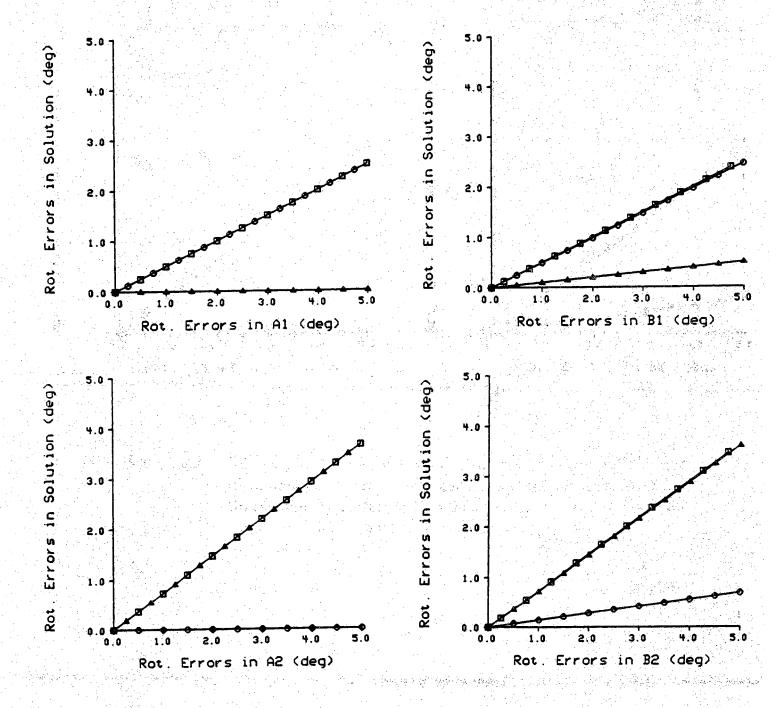
Figure 6.3. Rotational noise sensitivities due to rotational perturbations of robot motion measurements and sensor motion measurements. Errors due to perturbations about the x, y, and z axes are marked by  $\Box$ ,  $\bigcirc$ , and  $\Delta$ , respectively.
