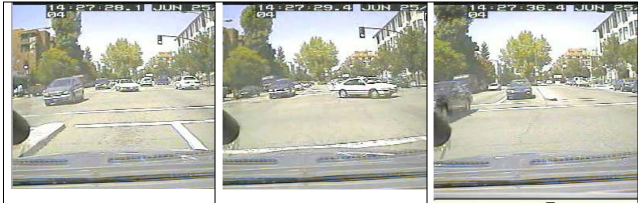
Figure 2-42. Example of a platoon clearing the intersection.
