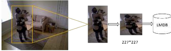
Figure 2. Image Preprocessing. Bounding box regions containing humans are extracted using OpenNI, re-scaled to 227 \times 227 pixels and normalised before encoding them via an LMDB database.
