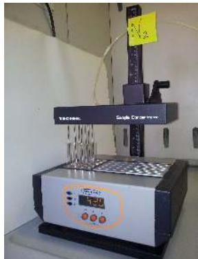
Figure 1. Sample concentration. Evaporation is increased by passing an inert gas (N 2 ) over the surface of the sample to remove the solvent. The gas travels through the gas chamber to the samples via the needles.
