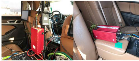
FIGURE 12. Test vehicle with RT3002 and RT-Range.
