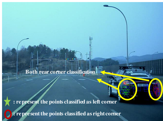
FIGURE 9. Classification result for both vehicle rear corner parts.
