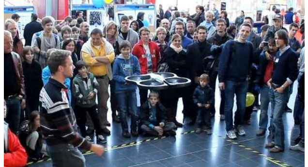
Fig. 1. A low-cost quadcopter navigates in unstructured environments using the front camera as its main sensor. The quadcopter is able to hold a position, fly figures with absolute scale, and recover from temporary tracking loss. Picture taken at the TUM open day.
