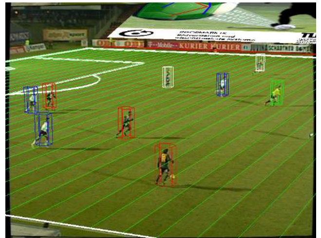
Figure 2: Output of the visual perception. The players and the ball in the camera view are detected. The players are labelled with respect to the team they belong to. For each player, the referee, and the ball the \langle x, y \rangle position is estimated.
