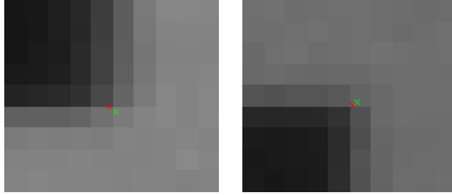
Fig. 3.4: Typical corner detection images, enlarged by a factor 20. The green cross marks the LI corner position, the red cross the SP corner position. Left: High resolution image. Right: Low resolution image.
