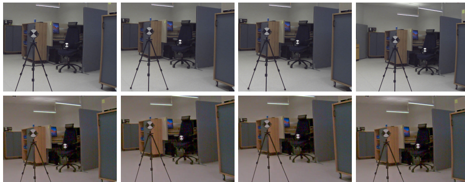
Fig. 4. The first column shows two images of two cameras, axis223m and axisp3364 , respectively. In the second and third columns, the undistortion looks to be visually removed for both D(1,0) [14], and D(3,0) [14]. Our method correctly detects D(1,0) [14] as incorrect for both cameras (Tables 2 and 3). The undistorted images in the fourth column are visually similar to their original, but this is not detected. For more details, see Section 4.2.
