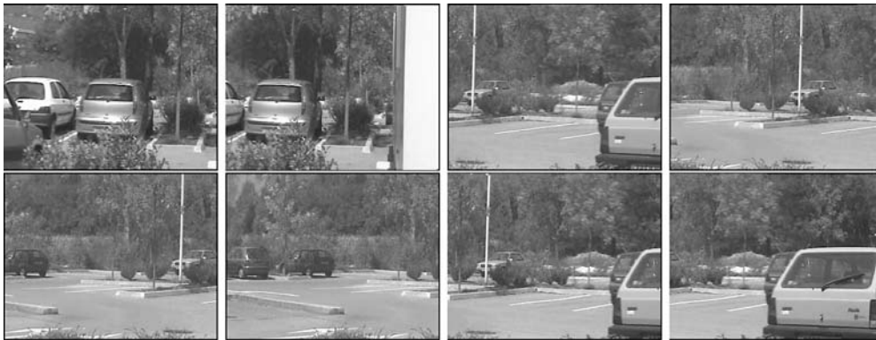
Fig. 9 The foreground pixels were removed from the image sequence and replaced by background using the image-to-image homographies
