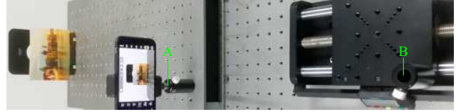
Figure 5. Acquisition strategy for the smartphone version of City100. Translating the smartphone away from a subject (from A to B), the effective resolution is decreased due to the enlarged FoV (R-V degradation).
