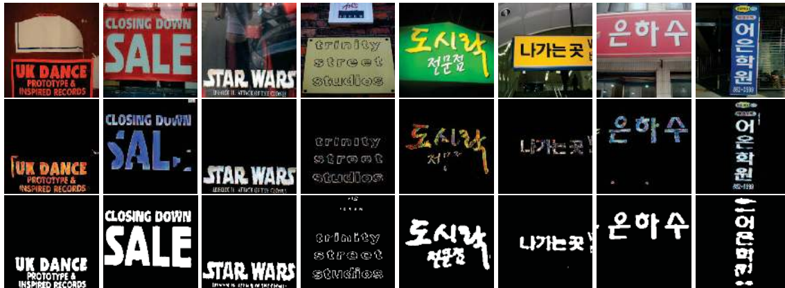
Figure 4. Qualitative results of English (first four columns) from ICDAR2013 dataset and Korean (fifth through eighth columns) from KAIST dataset. Each column shows the input image, output of CycleGAN trained in an unsupervised manner, and DCNN text segmentation based on DeepLabV3+ trained in a supervised manner. Korean text has been segmented in zero-shot learning, i.e. the trained models have never seen the Korean text images. Best viewed in color.
