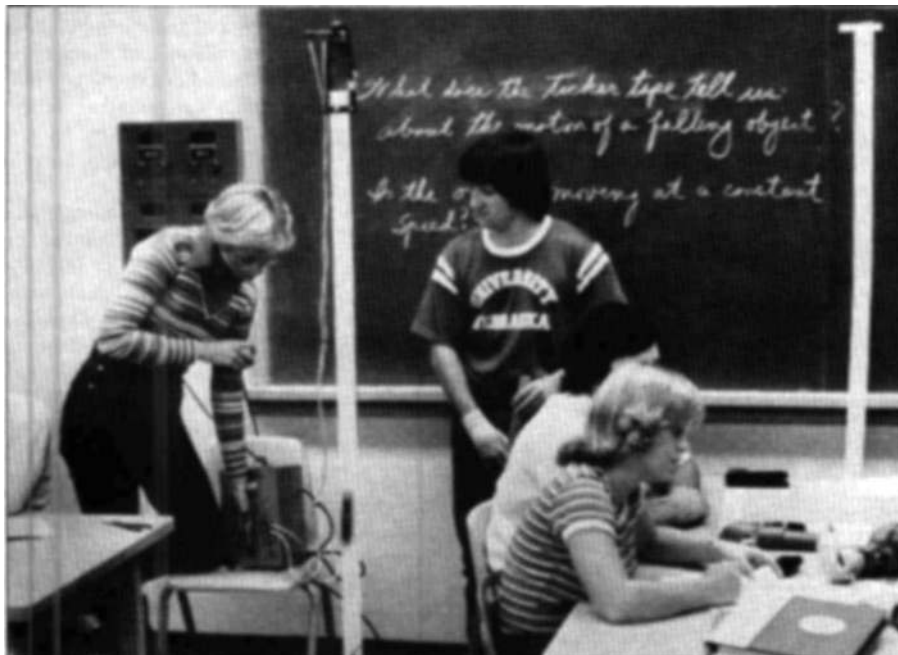
Sparks mark the position of the falling object on the ticker tape. The dot patterns can not be analysed readily by that third of US adolescents and adults who use only concrete reasoning.
