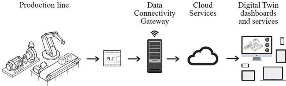
Fig. 2. Structure of condition monitoring system
