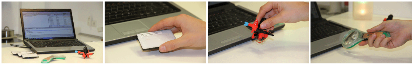
Figure 11. An exemplary workplace equipped with CapNFC-enabled objects for symbolic access to a very specific set of computer functionality. The transceiver is connected to the PC, having a receiver electrode placed under the user's desk.
