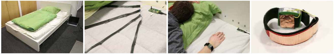
Figure 16. A bed that is able to receive messages from multiple body-worn sensors, for example a wrist-worn accelerometer. The accelerometer is grounded using ground-coupling by touch (inner electrode) and transmits its sensor values to the bed (outer electrode).
