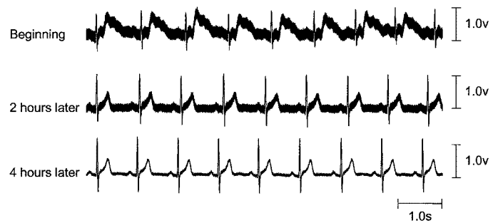
Fig. 6. Long-term recordings using the present device from the dorsum with an inserted cotton sheet 395 \mu\text{m} thick. S/N ratio of the recordings after 4 h was as good or better than that at the 4-h point. The room temperature was 21^\circ\text{C} and the relative humidity was 24%.
