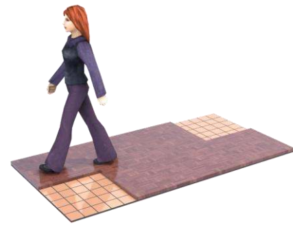
FIGURE 2. The structure of the floor. The floor can be topped with any non-conductive flooring material such as wood, vinyl or carpet.
