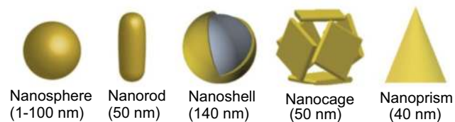
Figure 1 Different shapes of gold nanoparticles used in biomedical applications. Reprinted from Journal of Experimental & Clinical Medicine , 6, Ajnai G, Chiu A, Kan T, Cheng C-C, Tsai T-H, Chang J, Trends of gold nanoparticle-based drug delivery system in cancer therapy, pages 172-178, Copyright (2014) with permission from Elsevier. 47
