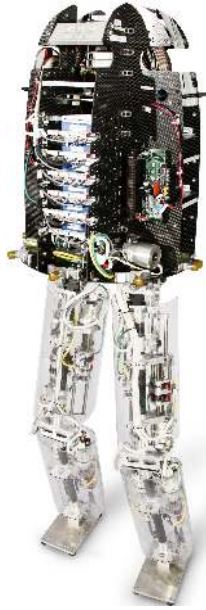
Fig. 1. M2V2, a twelve degree of freedom lower-body humanoid robot. The robot uses twelve identical Series Elastic Actuators in each of its joints. There are three degrees of freedom at each hip, one at each knee, and two at each ankle.
