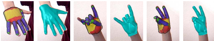
Fig. 2. Qualitative comparison with [27]. Each image pair corresponds to the pose estimate of the FORTH tracker (left) and our tracker (right)
