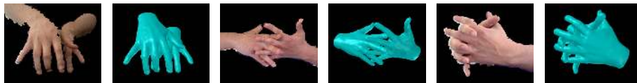
Fig. 1. Qualitative results of our pipeline. Each pair shows the aligned RGB and depth input maps after depth thresholding, along with the pose estimate output
