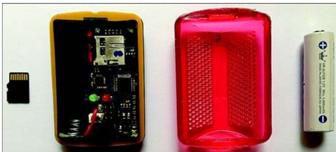
Figure 1. Configuration of NIGHT-Recorder consisting of five modules: microcontroller, power management module, sensor module, real-time clock module, and data storage module. It is powered by single AA battery (1,000 mA·h), and data are stored on 1 GB secure digital memory card.
