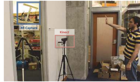
Figure 12—Tracking the Human Hand Through Walls. RF-Capture tracks the subject’s palm through a wall while the Kinect tracks it in line-of-sight.
