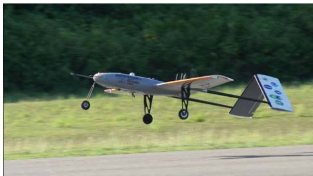
Fig. 2. ACR Manta autonomous unmanned aerial vehicle carrying aerosol-radiation payload landing in the Maldives.
