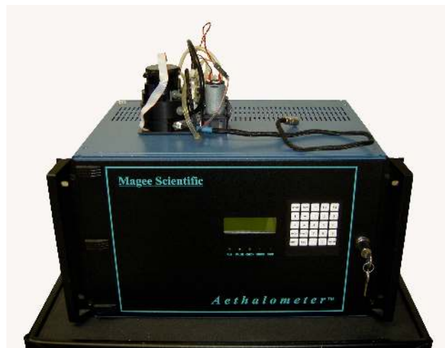
Fig. 3. Absorption photometer developed for deployment on AUAVs sitting atop the original, commercial, 19" rack-mount instrument (Magee Scientific AE-31 Aethalometer).
