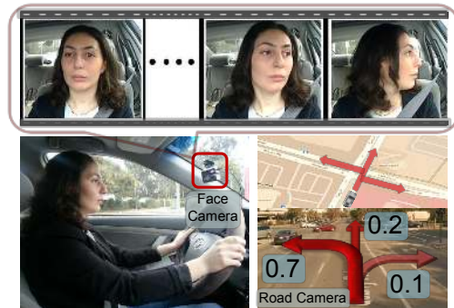
Figure 1: Anticipating maneuvers. Our algorithm anticipates driving maneuvers performed a few seconds in the future. It uses information from multiple sources including videos, vehicle dynamics, GPS, and street maps to anticipate the probability of different future maneuvers.
