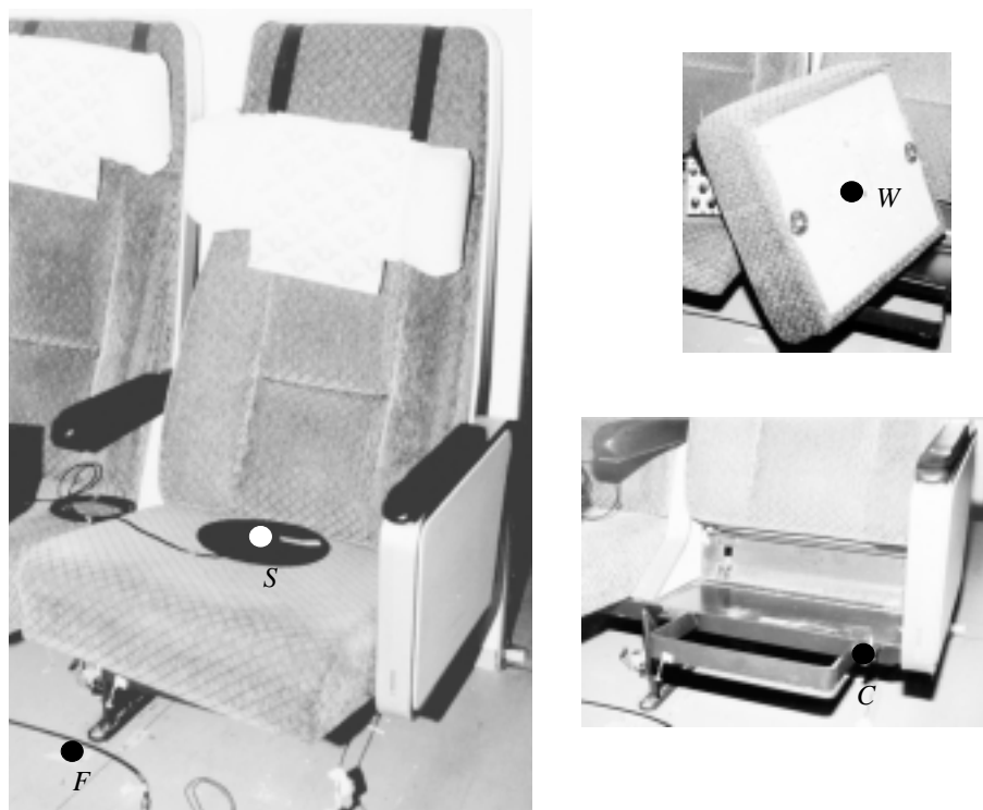
Figure 3-5 Four accelerometer positions on seat 24. (F) floor, (C) console, (W) wooden plate of seat pan and (S) seat pan, which is dismantled in the figures to the right.
