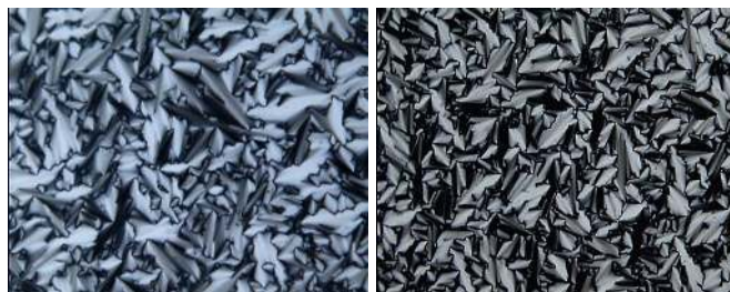
Figure 4: The fan-shaped texture of the SmA phase obtained upon slow cooling of the isotropic liquid of C_{13} -2d- \beta -Glc (left) and binary mixture C_{12} -2d- \alpha,\beta -Glc (1:1) (right).
