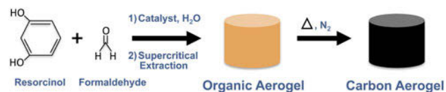
FIG. 1. Synthesis scheme for resorcinol–formaldehyde sol–gel path to CAs.
