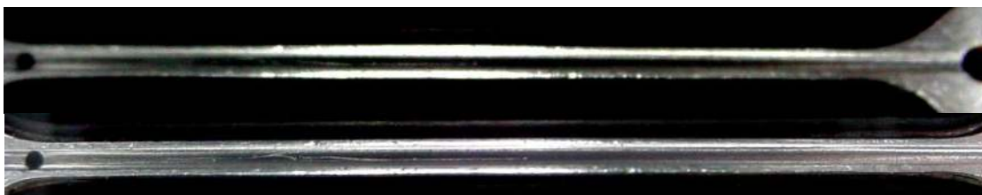
Figure 10(e). Flow pattern in test 56 (annular flow), where G=188 \text{ kg/(m}^2\text{s)} and x=0.79 .
