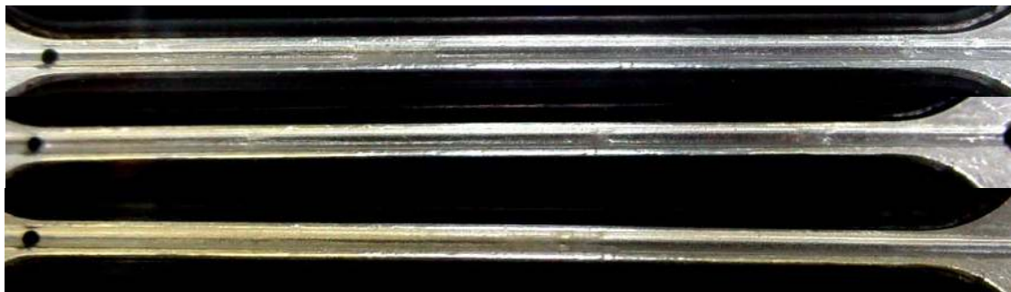
Figure 6(c). Flow pattern in test 3 (slug flow), where G=58 \text{ kg/(m}^2\text{s)} and x=0.48 .
