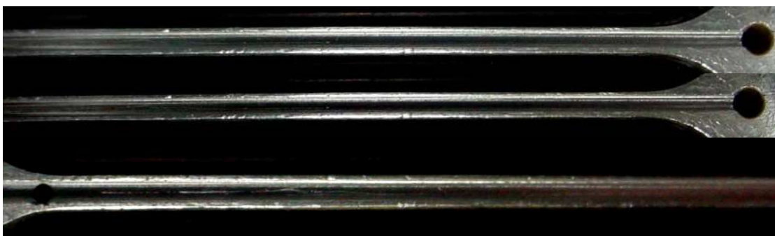
Figure 10(d). Flow pattern in test 55 (annular flow), where G=188 \text{ kg/(m}^2\text{s)} and x=0.67 .
