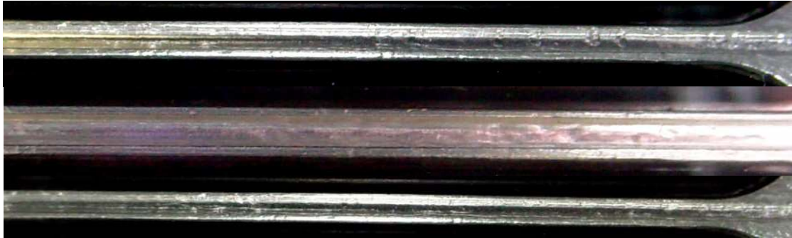
Figure 9(e). Flow pattern in test 45 (slug/annular flow), where G=149 \text{ kg/(m}^2\text{s)} and x=0.50 .
