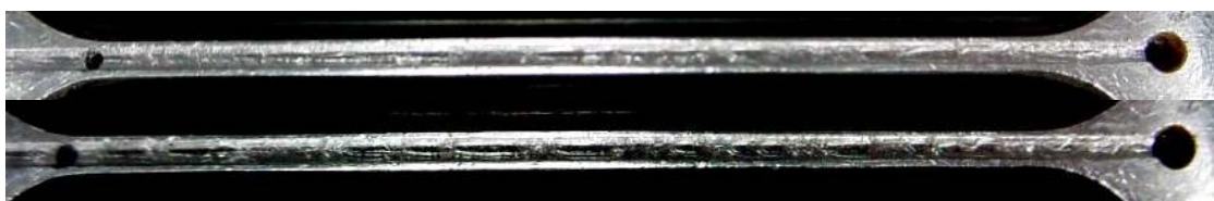
Figure 9(c). Flow pattern in test 41 (plug flow), where G=149 \text{ kg/(m}^2\text{s)} and x=0.25 .
