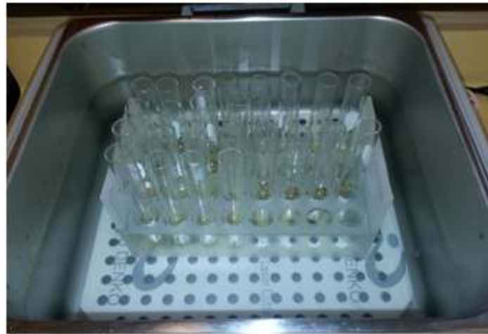
Figure 3. The set-up of the respirometers in the 30°C hot water bath.
