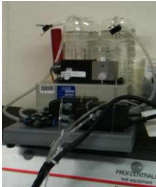
Figure 4.6 Initial apparatus to collect separate gas samples of expired and inspired air using two compartments of water
