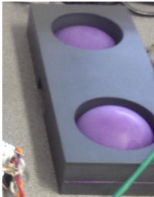
Figure 4.7 The modified apparatus to collect expired and inspired air samples using rubber balloon mechanism
