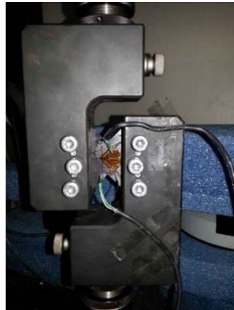
Fig. 2 V-notched shear test with a bonded rosette
