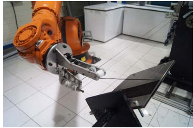
Fig. 1 Manufacturing of a flat unidirectional laminate by filament winding
