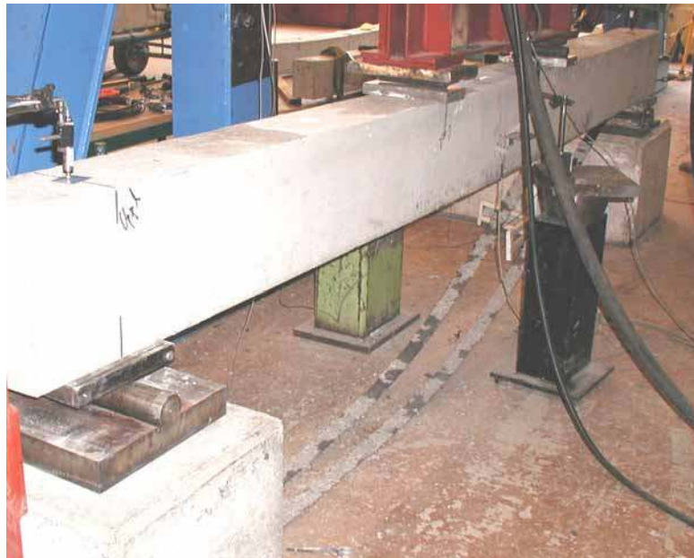
FIG. 13. Anchorage failure in the concrete for beam LSstat .
