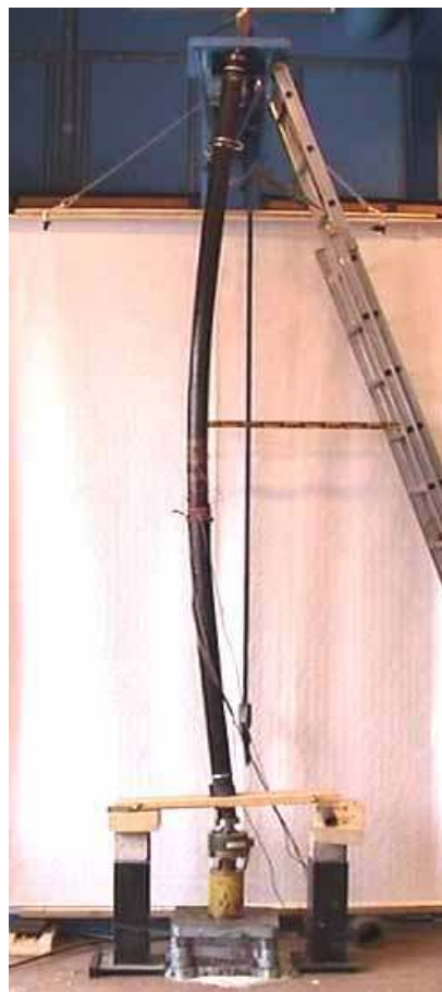
Fig. 6: Specimen C3600 after buckling.
