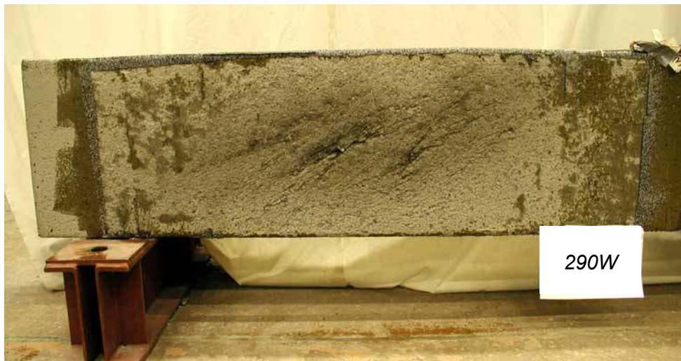
Fig. 14. Crack zone before ultimate shear failure
