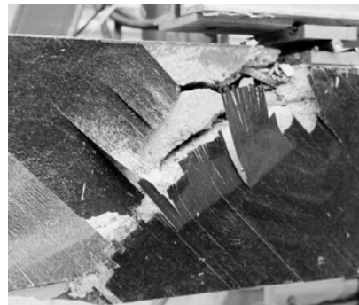
R, Fiber rupture
