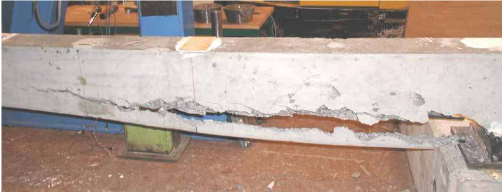
FIG. 15. Anchorage failure in the concrete for BMstat .
