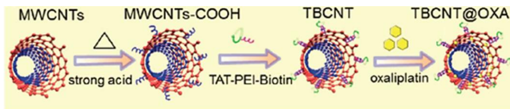
Figure 3. Synthetic scheme for TBCNT@OXA
