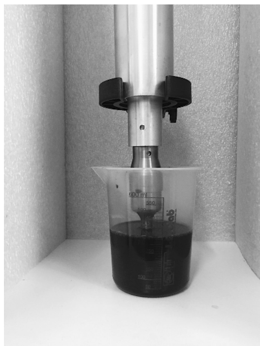
Figure 3. Sonication tip dispersing carbon nanotubes in aqueous solution [34] .
