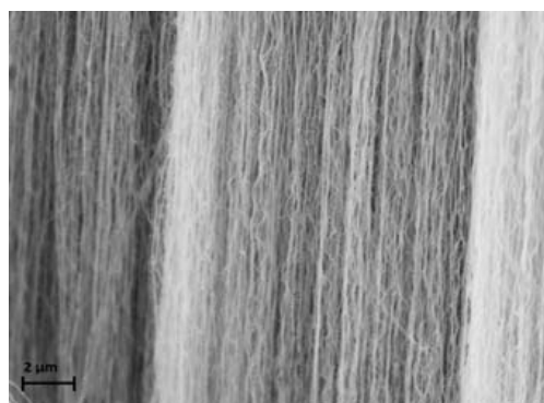
Fig. 6. SEM images of 550 \mu\text{m} tall carbon nanotube forest grown at Si coated by Fe catalyst showing the characteristic waviness of MWNT grown at higher temperature and reaction time.
