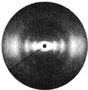
Fig. 3. Wide-angle X-ray diffraction picture of a single-wall carbon nanotube fiber drawn from a liquid-crystalline suspension in concentrated sulfuric acid. The pattern indicates high-quality alignment of the nanotubes with the fiber axis [124]
