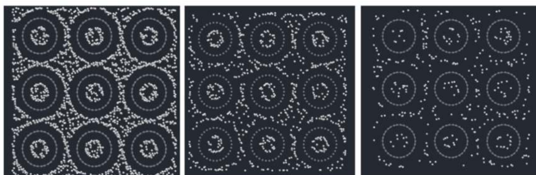
Figure 10. Hydrogen storage in nanotube bundles. Snapshots from grand canonical Monte Carlo simulations taken under 100 Bar pressure at 77 K (left), 175 K (middle), and 293 K (right) [173].
