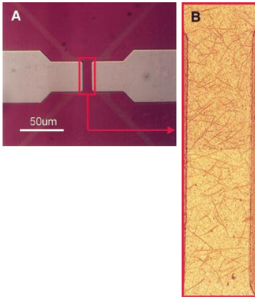
Fig. 12. CNTFET fabricated by Snow and co-workers at NRL in 2003 [57]. (A) Optical image of a CNTFET: Ti contacts were evaporated on top of a SWCNT film grown on thermal SiO 2 . Channel was 10 μm long. The Si substrate serves as a back gate. (B) Representative AFM image of a SWCNT network that shows multiple conduction pathways via interconnected CNTs.
