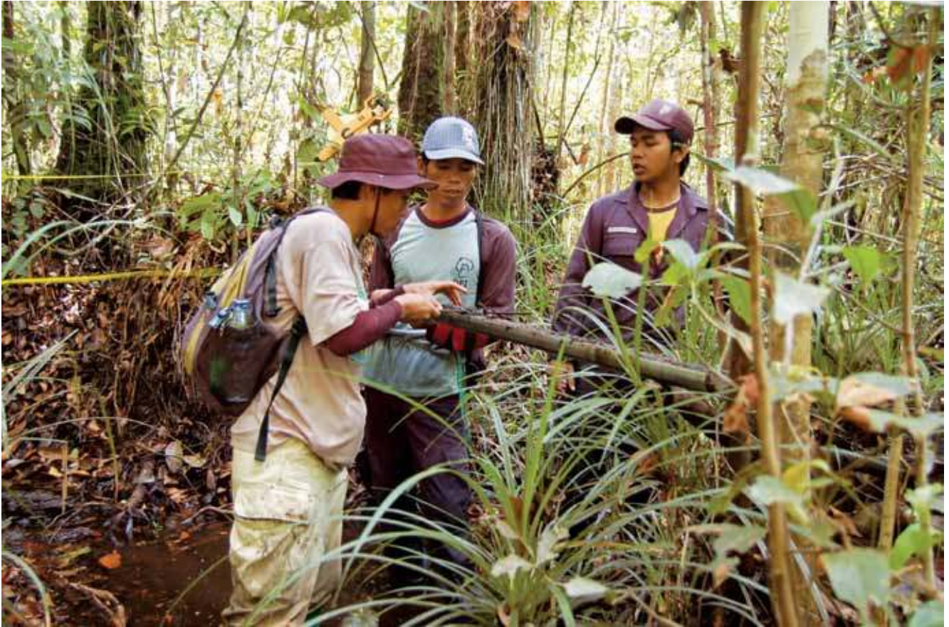
Our field team collects organic material and soil samples using a specially designed peat auger.
