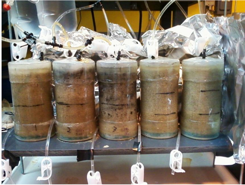
Figure 12a- Five acrylic sand columns are filled and sitting on a PVC platform. Some of the columns were interconnected depending on the column treatment.
