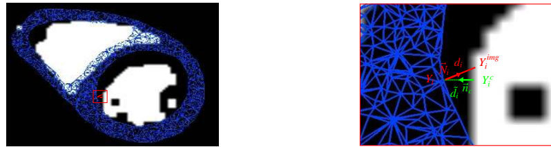
Figure 4: Distances \tilde{d}_i of the mesh to the blood pool (green) and d_i of the blood pool to the mesh (red).
