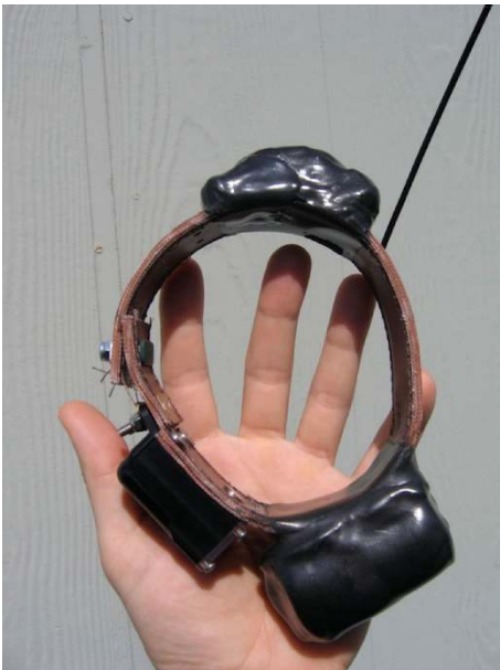
FIGURE 3: Deployed CARNIVORE node. This collar was deployed on a mountain lion. The CARNIVORE electronics are above, D-cell battery and VHF beacon are lower right, and a timed dropoff (SirTrack [17]) is lower left. VHF antenna can be seen exiting the collar upper right. The VHF beacon and dropoff use separate power supplies from the CARNIVORE platform. Components were assembled by Telemetry Solutions.
