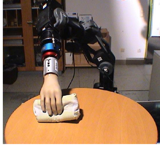
Fig. 1. DLR light-weight robot, generation II, using impedance control in a table wiping application.
