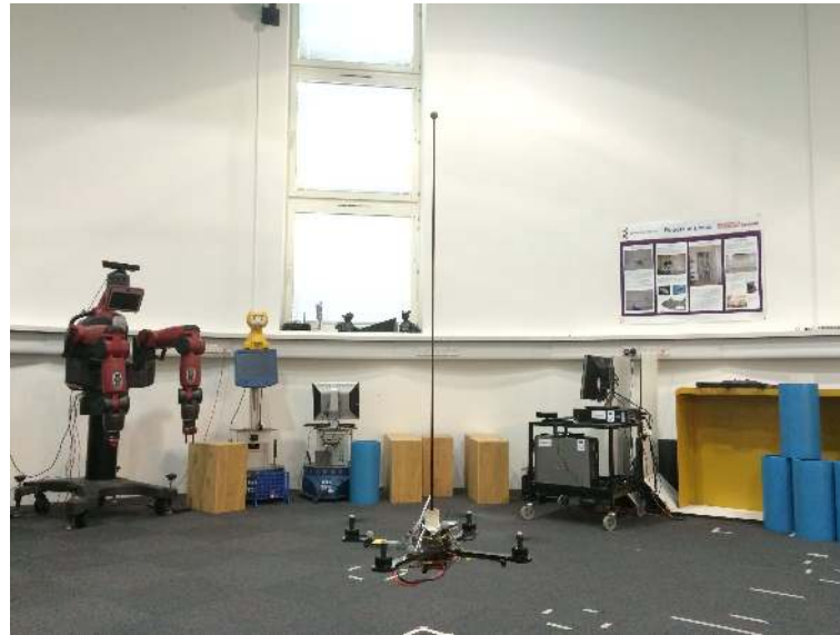
Figure 13. An inverted pendulum on a hovering quadrotor.
